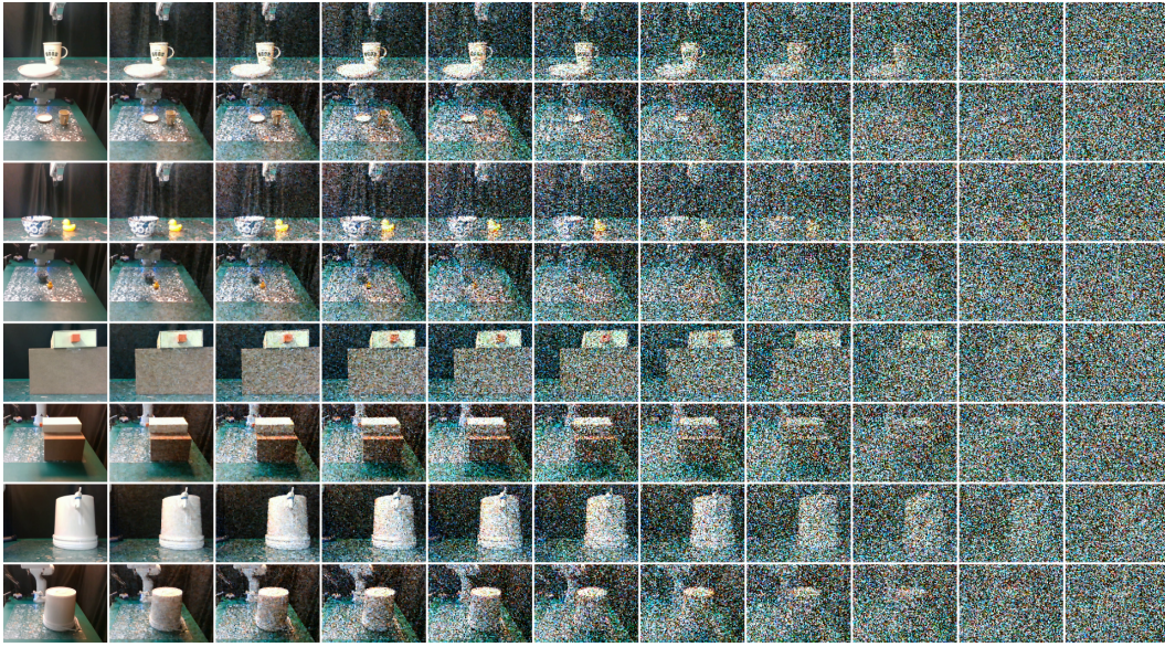
Figure 15: Realworld Inversion Results. Each task corresponds to two rows, with each representing a distinct camera view. The first column of each row is the original image, while the other columns are the DDPM inversion results. Starting from the second column, the diffusion steps are increased from 5 to 50, with the incremental step being 5.
